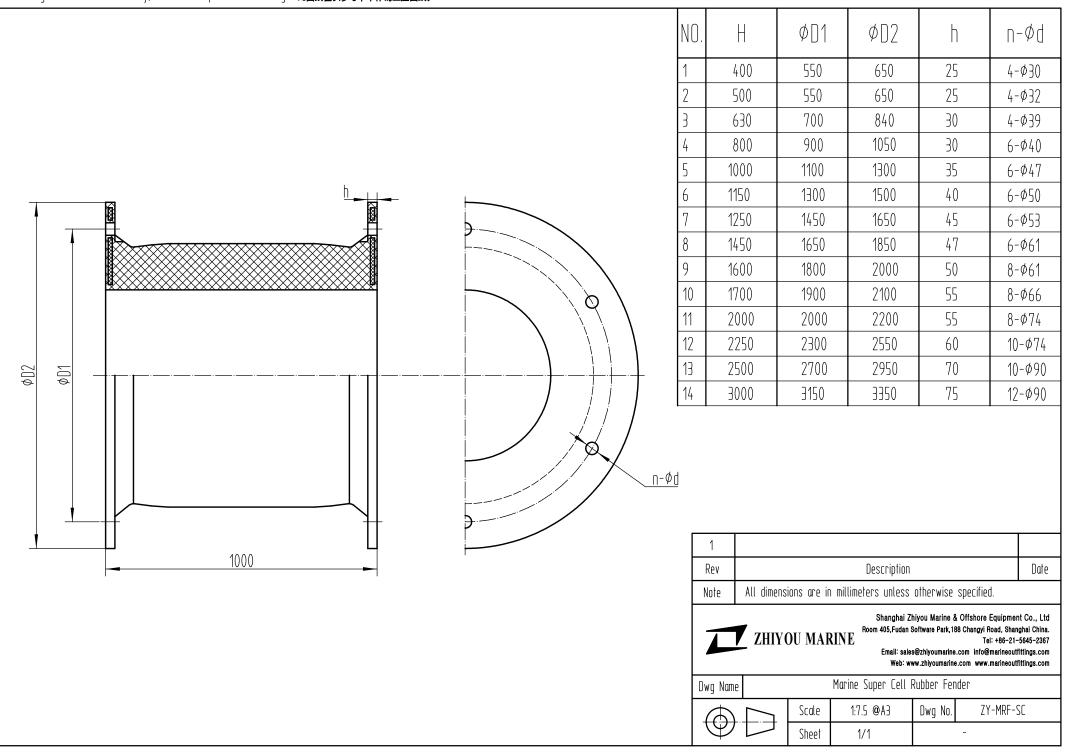
The drawings are for reference only, not used as production drawings. 此圖紙僅供參考,不作為生產圖紙。
